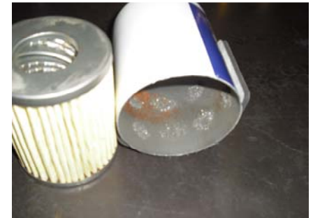
Circles inside above can is captured contamination from magnetic filtration.
